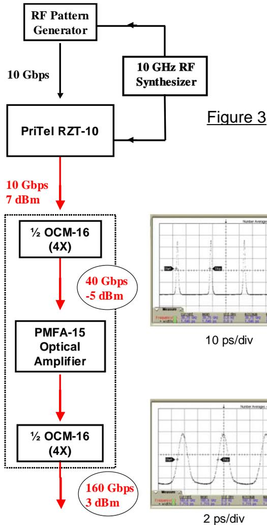
Figure 3 shows a typical application of the OCM-16 to a PriTel RZT-10 fiber laser. The electrical pattern data at 10 Gbps are delivered to the RZT-10, which uses an embedded data modulator to impress the electrical pattern on the 10 GHz optical clock stream.
